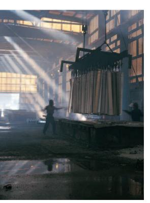
**Surface preparation** insures that the zinc will react properly with the steel. The preparation starts with caustic cleaning to remove organic contaminants such as dirt, grease and oil. Pickling then removes scale and rust followed by fluxing which removes oxides and prevents further oxides from forming on the surface of the steel. It also promotes bonding of the zinc to the steel surface.
